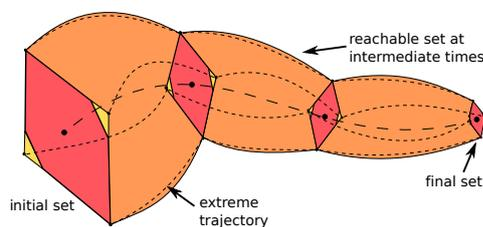
*Illustration of novel, set-based control approach from [1], where a formal control law for a set of initial states is obtained by interpolating the optimal solutions for single extreme states.*
